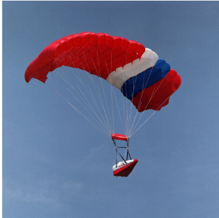
Figure 1.2 An example of a parafoil in flight. This photo is of the NASA SpaceWedge system, a precursor to the X-38 program. Photo courtesy of NASA Dryden Flight Research Center.
