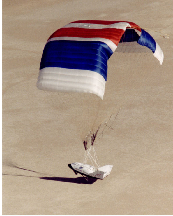
Figure 2.2 Side view of the X-38 Crew Return Vehicle just prior to touchdown. A large symmetric flap deflection can clearly be seen. Photo courtesy of NASA Dryden Flight Research Center.
