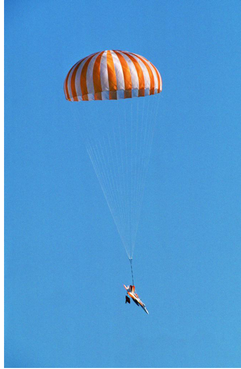
Figure 1.1 An example of a traditional non-gliding parachute. Photo courtesy of NASA Langley Research Center.
